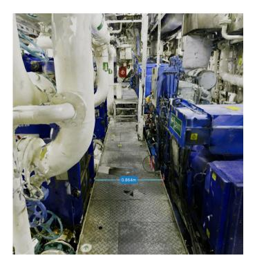
Every cabin, compartment, and engine space was intricately recorded in full 3D using the Leica RTC360 laser scanner. Subsequently, the scans were processed utilizing Leica Cyclone software before being uploaded as .E57 files to the quick and efficient Prevu3D software. Impressively, Prevu3D swiftly uploaded all
